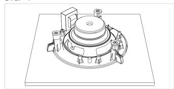
Fix the speaker in the provided opening by tightening the screws of the mounting clamps using a screw driver. A quarter turn will make the mounting clamps flip-out, locking the speaker in place. Tighten the screws for proper fixation of the speaker.
