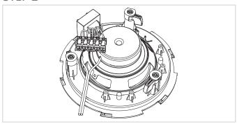
Connect the wires coming from the amplifier to the FastCon™ terminal block connector on the loudspeaker.
