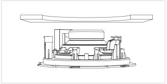
Make sure the mounting clamps are fully bended inwards, allowing the speaker fit through the cut-out. Insert the speaker to the opening.
